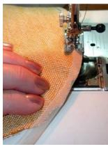
Note: Using the nylon tricot finish is important for a successful reverse flat-fell seam. Stretch the tricot during application, and force the curved edge of the hood to draw up so that the completed seam will fit smoothly into the contours of the hood. In addition, the tricot finish will give you something to grab onto as you fold the seam allowance under to create the flat fell. Without it, you run the risk of raveling fabric and a distorted seam.
