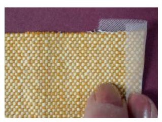
Insert fabric into the curl. Fold carefully so that the bottom half is wider than the top half. Fold nylon strip carefully over raw edge; do not pull or stretch.
