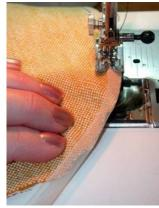
Note: Using the nylon tricot finish is important for a successful reverse flat-fell seam. Stretch the tricot during application, and force the curved edge of the hood to draw up so that the completed seam will fit smoothly into the contours of the hood. In addition, the tricot finish will give you something to grab onto as you fold the seam allowance under to create the flat
