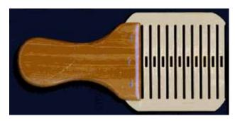
**Experience the speed of a warping** paddle. The combination of slots and holes allow warping multiple threads, from 2 - 20 ends at a time (depending on the brand). The hole and slot design allows formation of a warp cross and warp repeats are as
