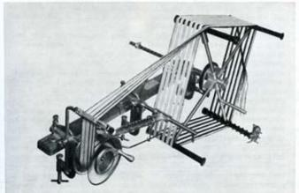
Warper and Beamer winding 2 inch spool section from reel
