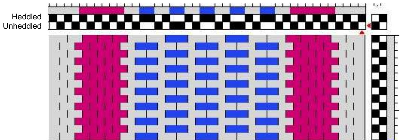
Follow the draft above to pre-warp the loom. The color sequence and placement are critical to a successful class. The color bar across the top of the draft indicates the color for each warp thread. The first thread on the left is heddled, and is pictured as light
