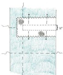
• Cut a rectangular patch of **fusible woven interfacing**, 2 %"(6cm) long and 1 ½"(3.8cm) wide. <a href="https://www.weaversew.com/shop/pellon-shape-flex.html">https://www.weaversew.com/shop/pellon-shape-flex.html</a> and pin securely with **right sides together** (glue side facing up) to the facing, centering over the basted placement line and extending past the stop line %"(1cm).
