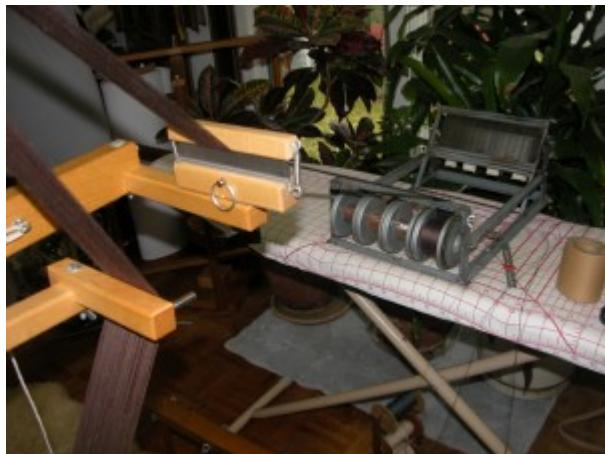
using the 20 dent reed, which meant the real width here was only 1 1/2". Then I beamed one of the spools directly off the AVL mill, right onto the back beam of the loom, which is missing its entire castle housing because my son has it apart on my cutting table. You can see the band of thread coming through the 20 dent reed.
