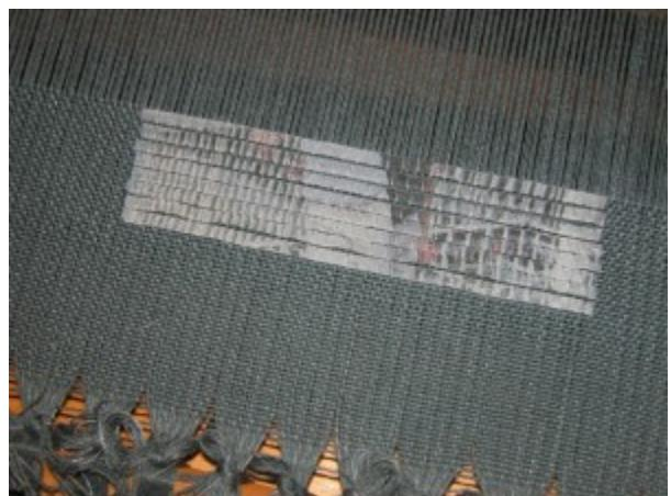
Here is a shot of the actual linen cloth, it is pretty fine, the linen is about the weight of a 20/2, and sleyed two per dent, I have 30 ends per inch, not counting the tie down threads.
