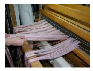
The term "front to back" denotes a way of warping the loom by sleving the reed first and then the heddles, followed by beaming. There are lots of tips and tricks to make this method fool proof, yielding perfectly tensioned and accurate warps every time. Step-by-step presentation.
